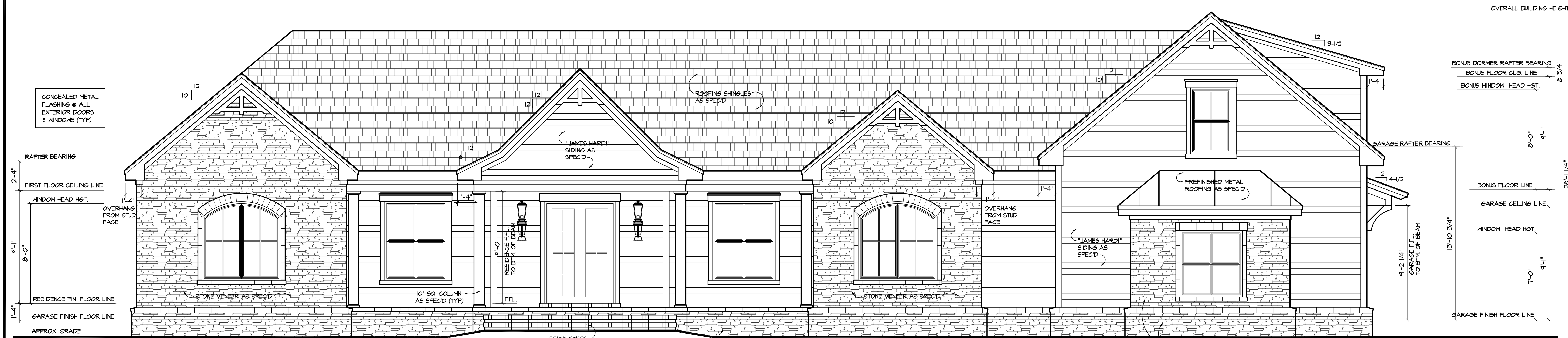
FRONT ELEVATION-C SCALE: 1/4" = 1'-0"
